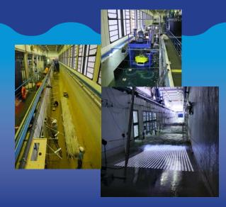
The windows along the flume and the pumping and filtering system, that keeps the water clean, allow non-intrusive optical observation techniques to be used in a wide range of experimental arrangements on a close- to-real scale.
